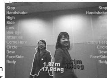
Recognition of the distance and direction of movement of multiple objects
